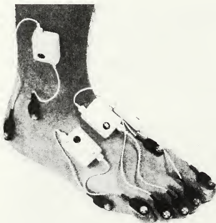
Figure 5. CODA mpx30 active, light-emitting diode (LED) motion markers placed on the foot of a subject. The sequentially strobed markers enable them to be placed close together without merging in the cameras. Each battery pack provides the power for two markers and houses circuitry to receive an infrared (IR) strobe signal. Photograph is courtesy of Charnwood Dynamics and is used with permission.
